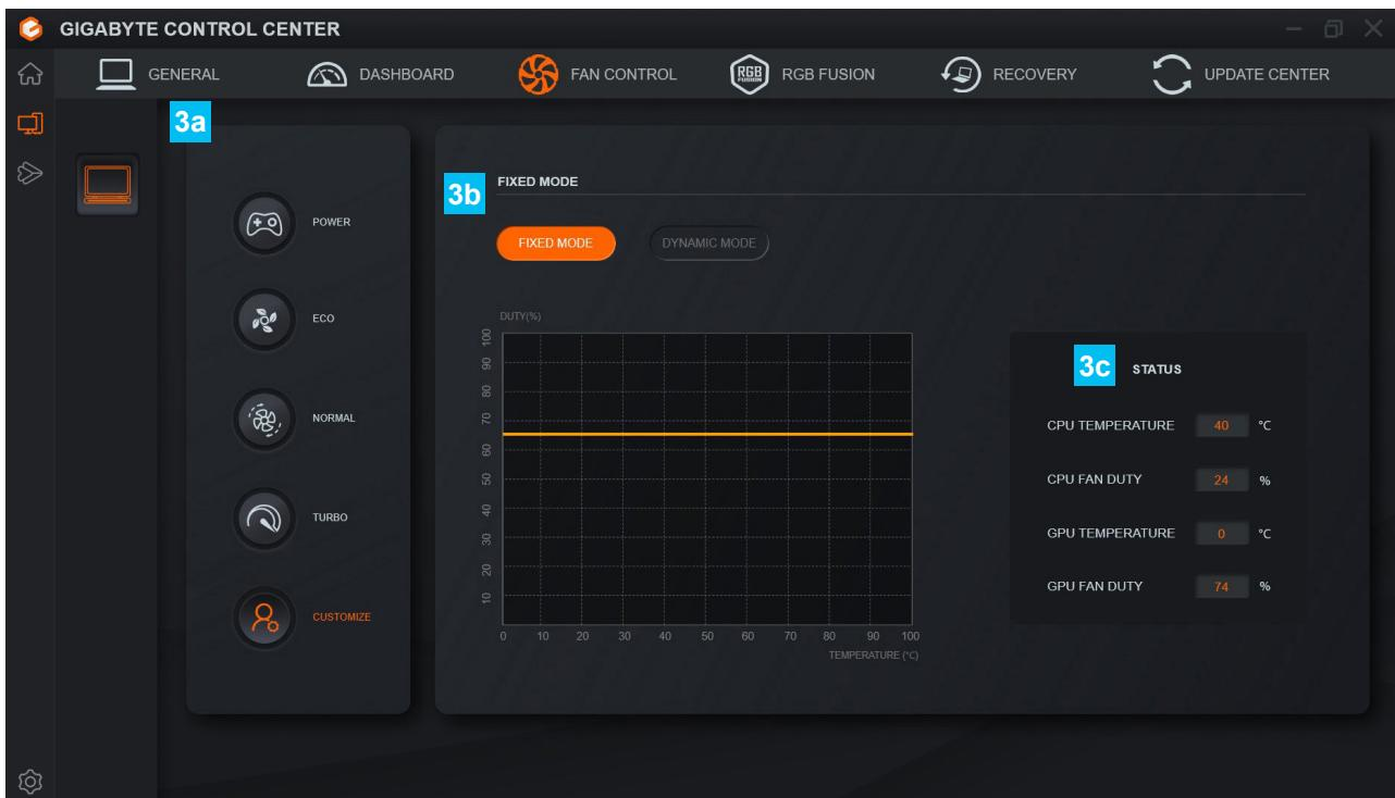
**3a** **Fan control** (Power Mode / Energy-Saving Mode / Normal Mode / Turbo Mode / Customized Mode).
